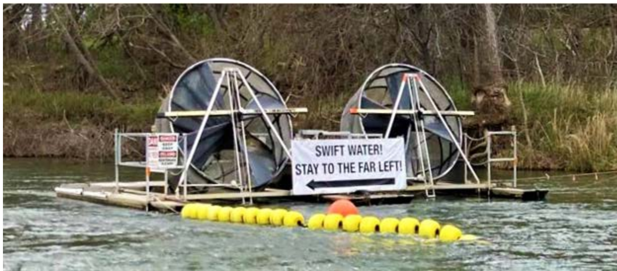
Figure 3: The two north channel 8-foot RSTs, Trap 8.1 (right) and Trap 8.2 (left), on the lower American River downstream of the Watt Avenue Bridge.
